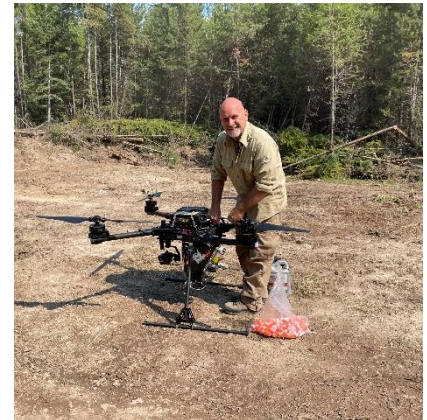
Drone with "ping pong balls" for ignition by the 3710 road – Amy Ando
